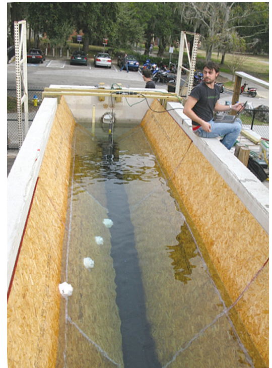
Scaled physical model to optimize FAA pond design criteria at the University of Florida, Gainesville.
