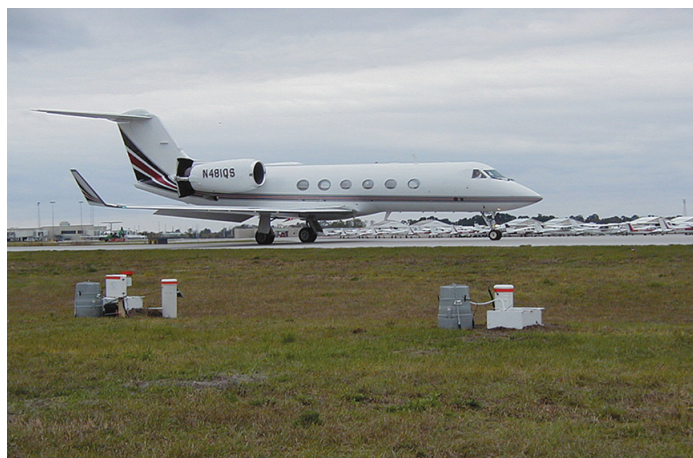
A paired stormwater sample collection system for testing water quality directly from the runway pavement and overland flow away from the pavement at Orlando Sanford International Airport.
