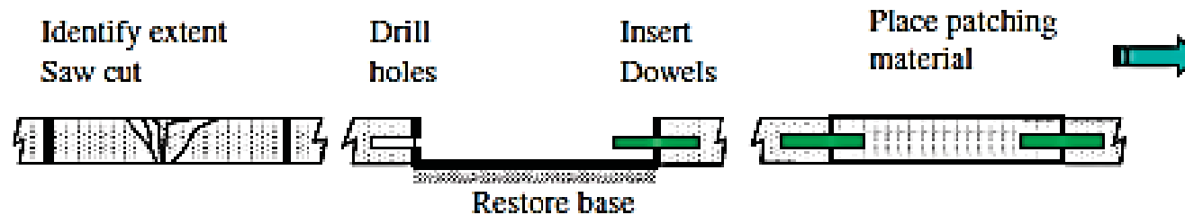
Sequence of Operation of Full-depth Repair of PCC Pavements
