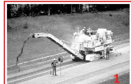
FIGURE 14-5 Typical milling machine.
