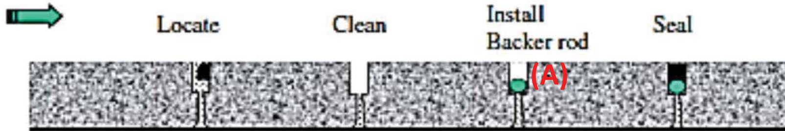
Sequence of Sealing Joints and Cracks in PCC Pavements
