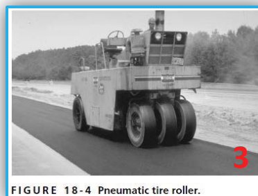
FIGURE 18-4 Pneumatic tire roller.
