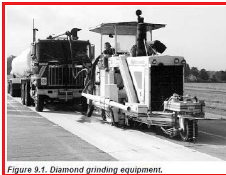
Figure 9.1. Diamond grinding equipment.
