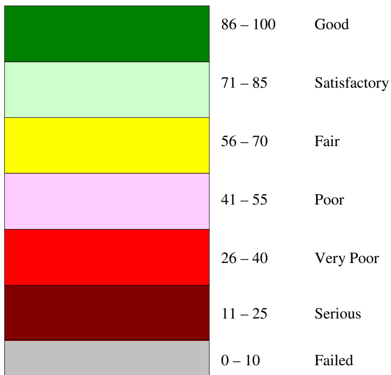
Figure 1-2: PCI Rating Scale
