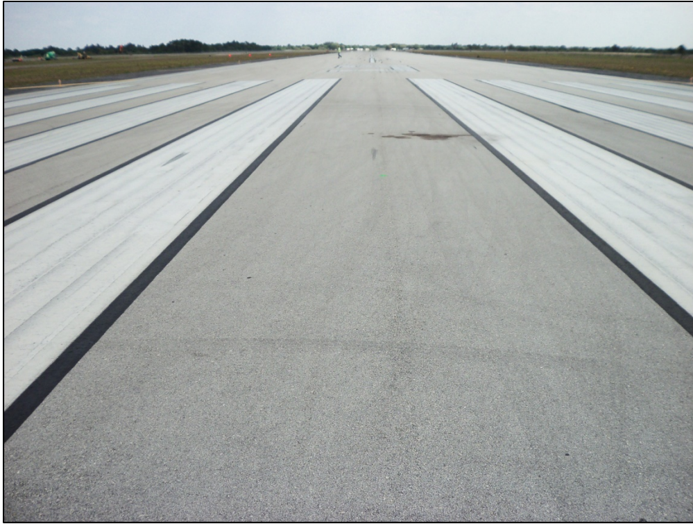
Runway 5-23, Section 6105, Sample Unit 101 – Low severity (48) Longitudinal Cracking, (49) Oil Spillage, and low severity (52) Weathering and Raveling
