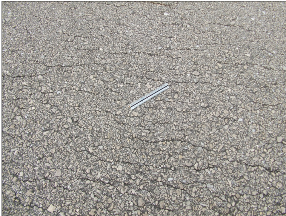
Taxiway Mike, Section 1330, Sample Unit 100 – Medium severity (52) Weathering and Raveling; low severity (55) Slippage Cracking.
