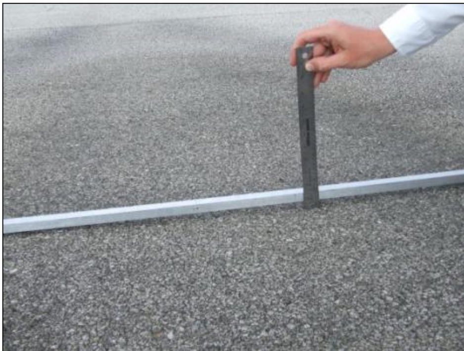
Taxiway Bravo 3, Section 260, Sample Unit 301 – Medium severity (45) Depression, low severity (48) Longitudinal and Transverse Cracking, low severity (50) Patching, low severity (52) Weathering and Raveling.
