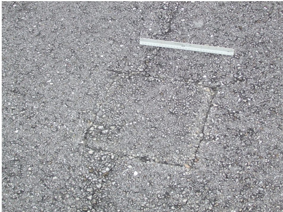
Apron, Section 4105, Sample Unit 202 – Low severity (48) Longitudinal and Transverse Cracking, low severity (50) Patching
