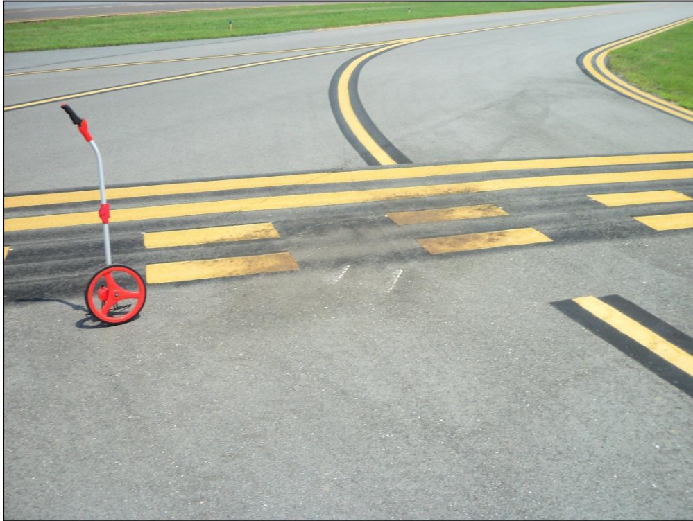
Taxiway A1, Section 115, Sample Unit 201 – Low Severity (45) Depression
