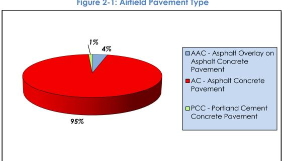
Figure 2-1: Airfield Pavement Type
