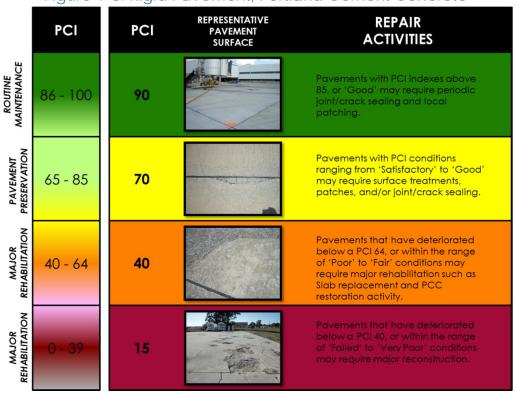
Using the ASTM D 5340-11 standard seven qualitative ranges, the SAPMP provides a PCI value and a standard qualitative condition rating for the pavement facilities inspected.
