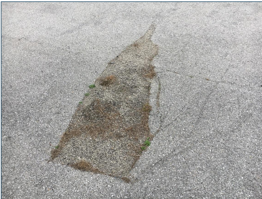
West Apron, Section 4115, Sample Unit 102 – High Severity (50) Patching, Low Severity (52) Raveling
