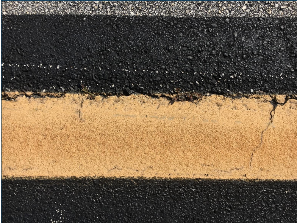
Taxiway A, Section 105, Sample Unit 121 – Low Severity (48) Longitudinal and Transverse Cracking, Low Severity (52) Raveling, Low Severity (57) Weathering
