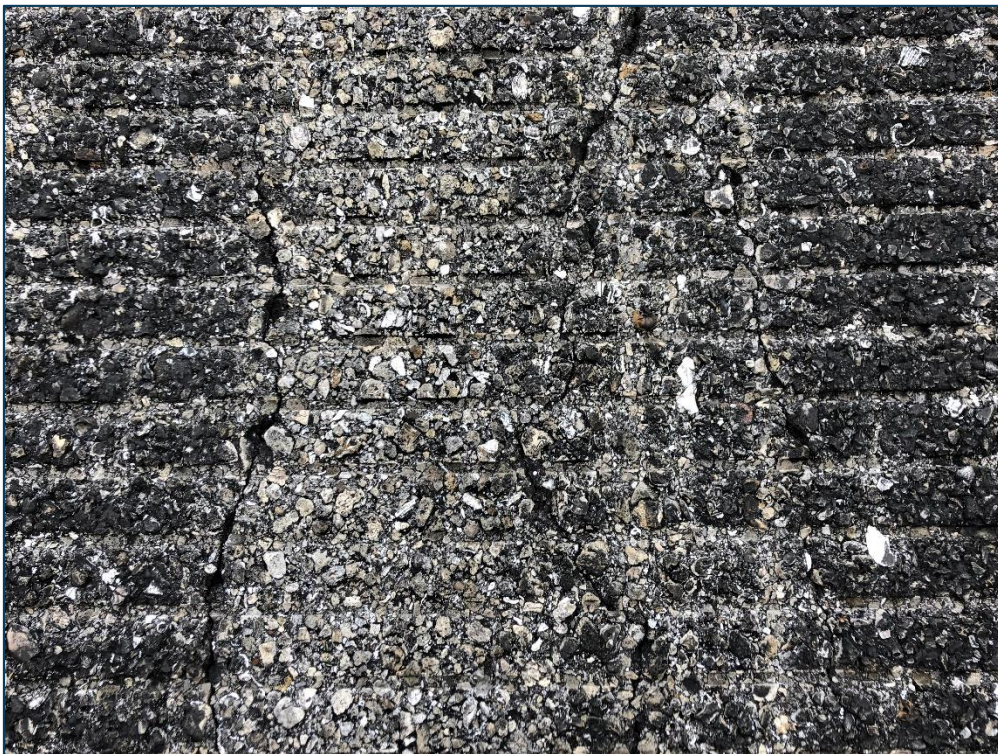
RW 4-22, Section 6105, Sample Unit313 - Low Severity (41) Alligator Cracking, Low Severity (52) Raveling, and Medium Severity (57) Weathering
