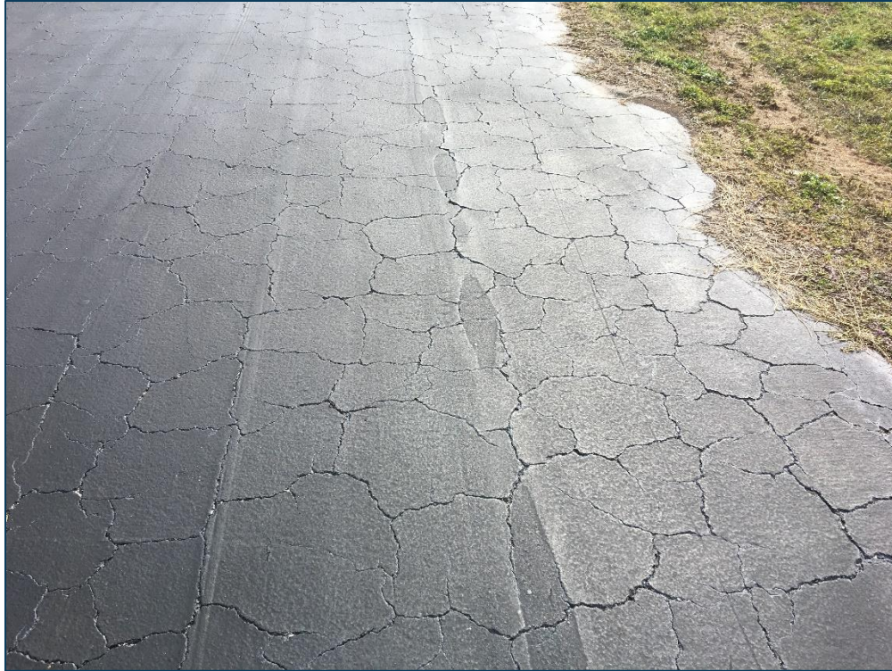
AP CENTER, Section 4410, Sample Unit 301 - Low Severity (43) Block Cracking, Medium Severity (43) Block Cracking, and Low Severity (57) Weathering
