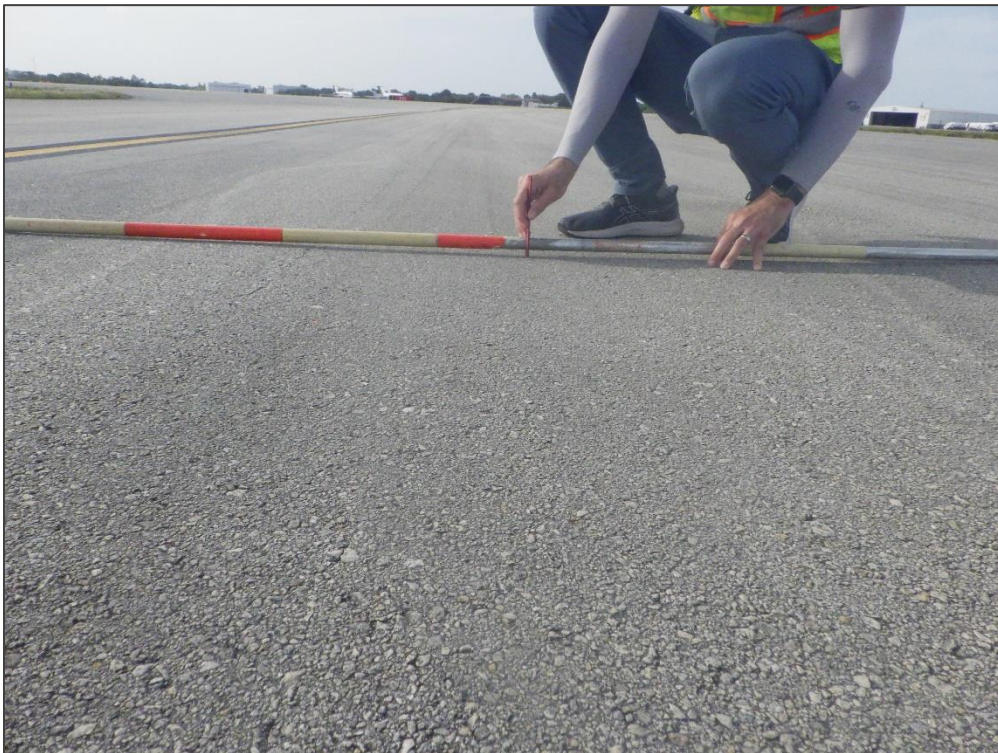
TW U, Section 2105, Sample Unit 103 – Rutting
