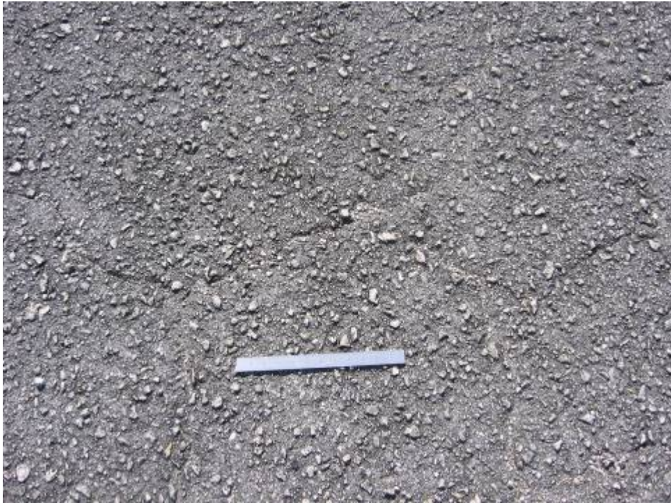
RW 14-32 Section 6220 SU 172: Low Severity Weathering (October 11, 2006)
