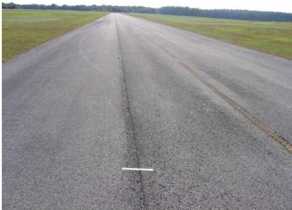
TW B Section 205 SU 115: Low Severity L/T Cracking (October 11, 2006)
