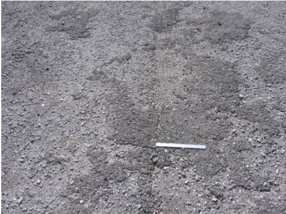
RW 14-32 Section 6220 SU 188: Medium Severity Weathering (October 11, 2006)
