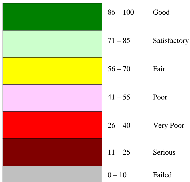
Figure 1-2: PCI Rating Scale
