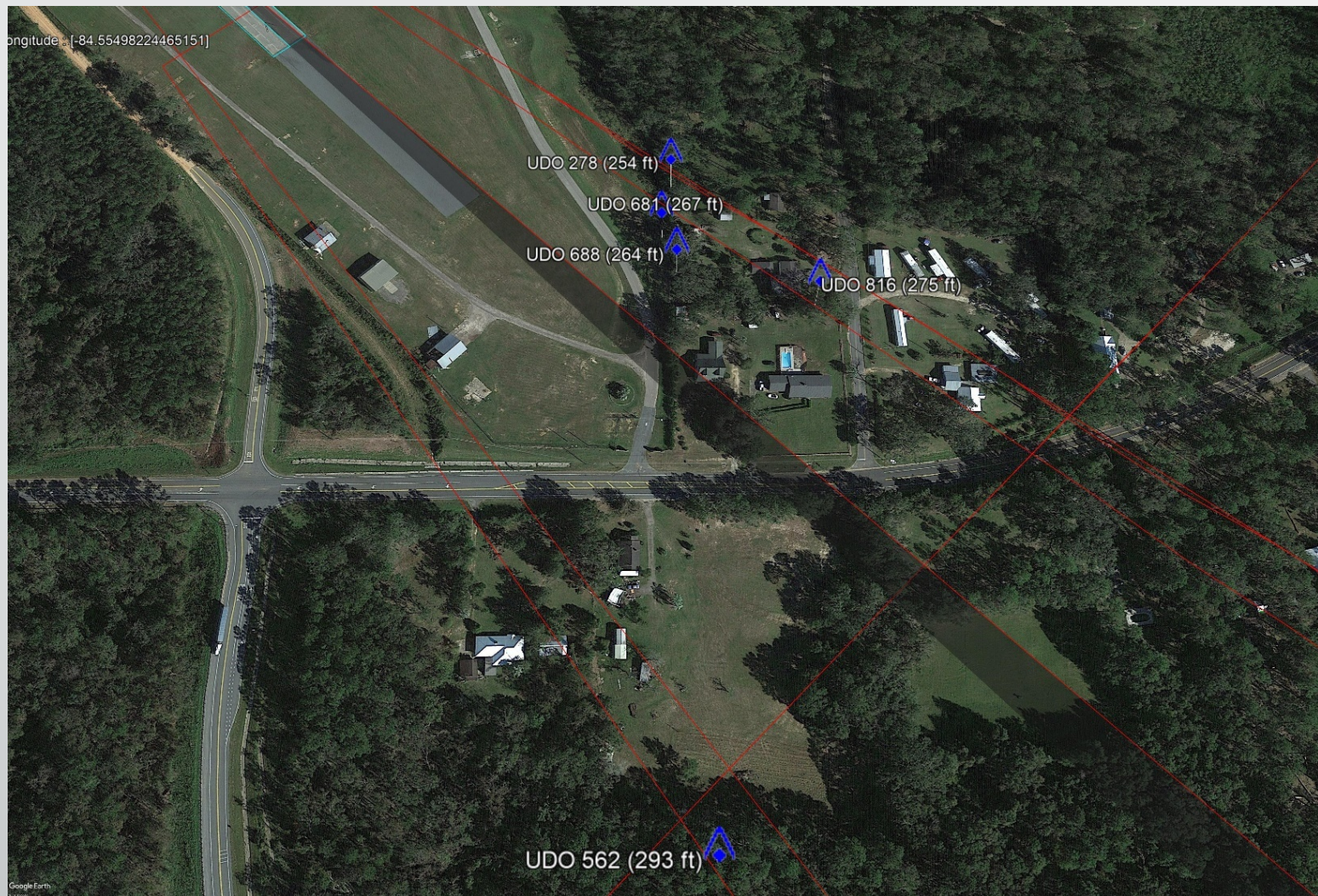
RWY 32 Final Segment - Visual Area - 20:1 Penetrating Obstacles
