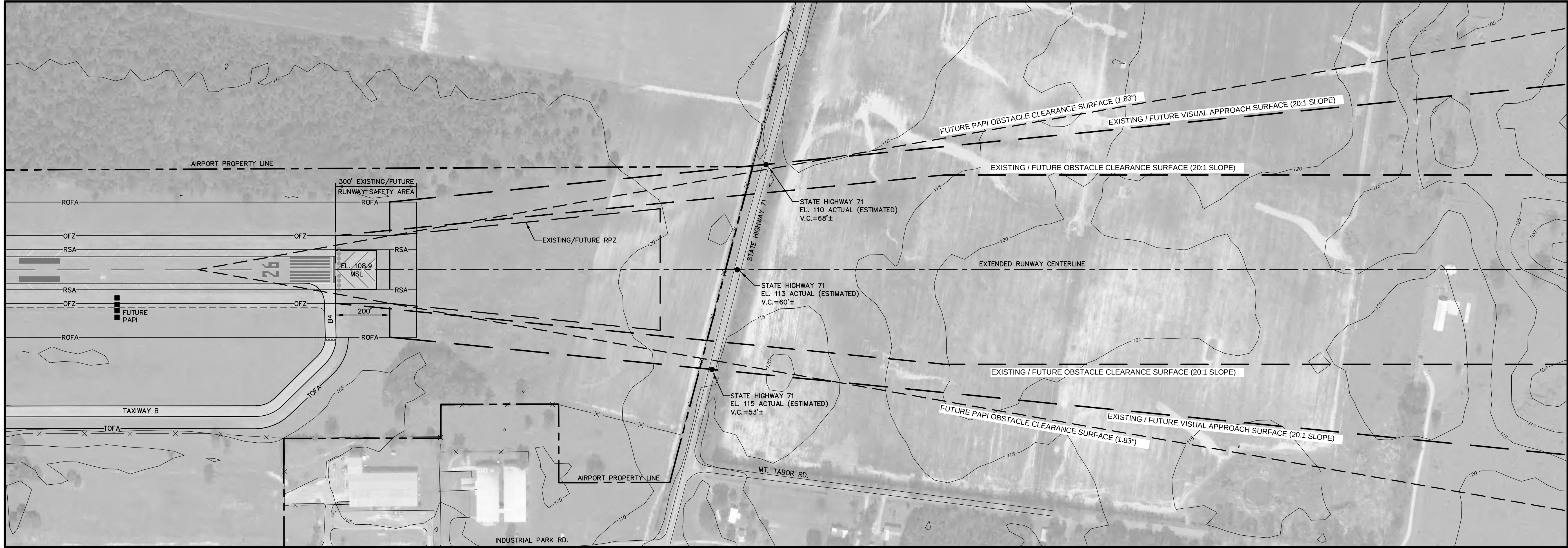
RUNWAY 26 INNER APPROACH SURFACE PLAN VIEW
