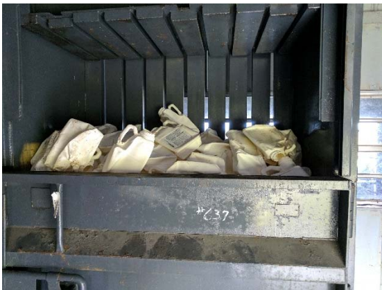
Figure 8: FFS Baler for HDPE Containers
