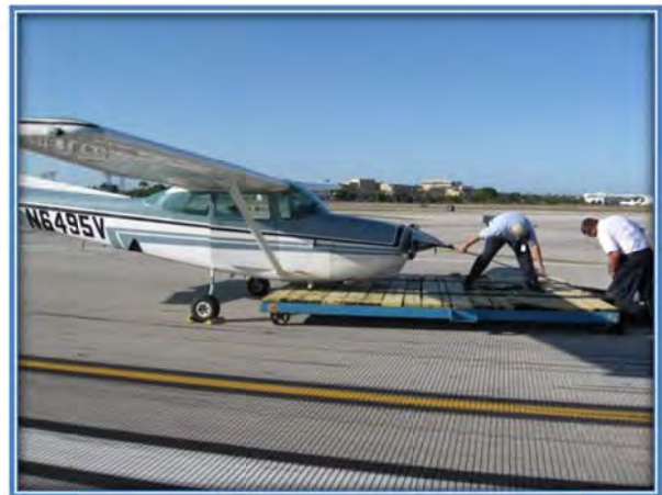
Figure 16: Wheel dolly being used to remove an aircraft
