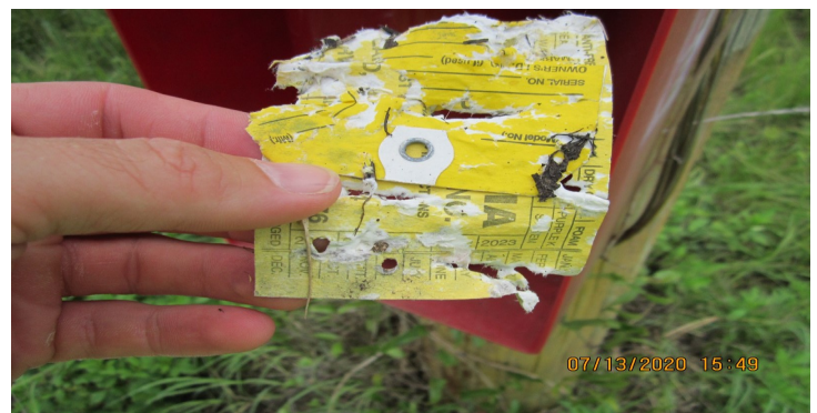
Example of a paper tag inspection label that fell off. It is highly recommended these labels be adhesive stickers.
