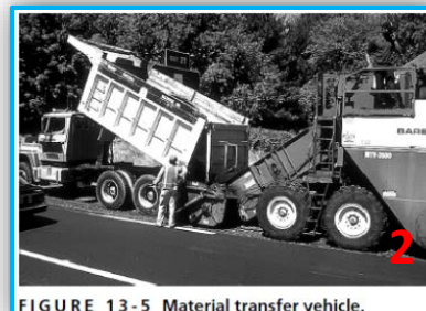
FIGURE 13-5 Material transfer vehicle.
