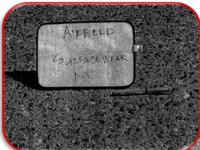
Medium-Severity Weathering (Surface Wear)
