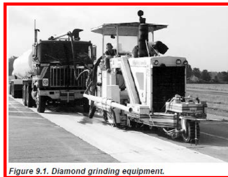
Figure 9.1. Diamond grinding equipment.
