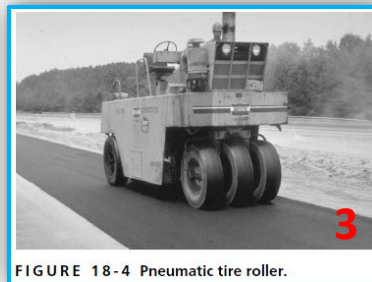
FIGURE 18-4 Pneumatic tire roller.
