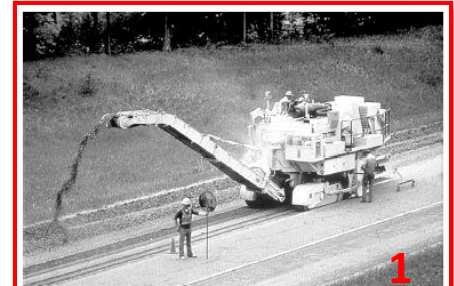
FIGURE 14-5 Typical milling machine.
