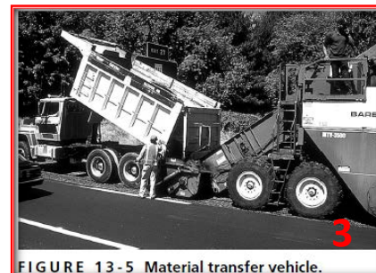
FIGURE 13-5 Material transfer vehicle.
